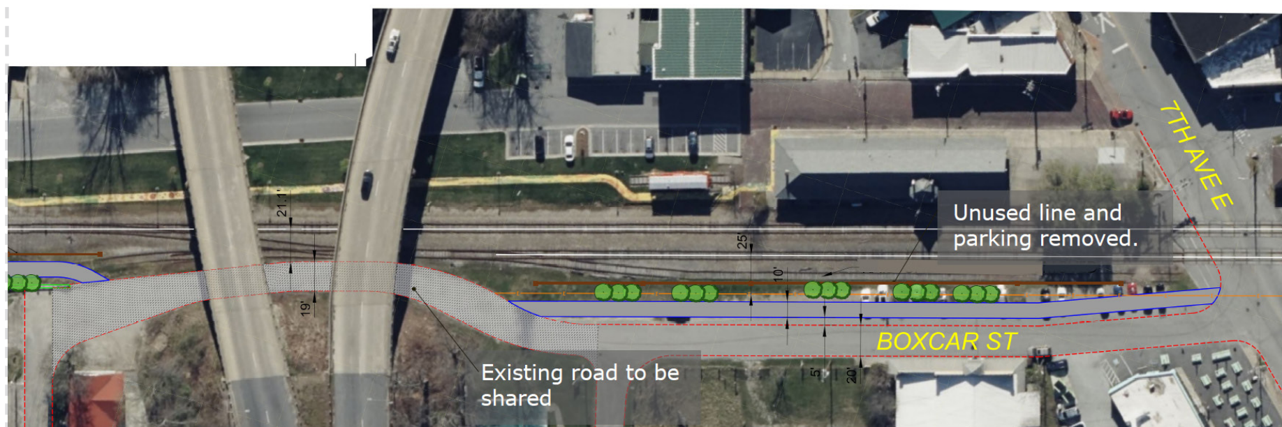
Image 41. Rail-with-Trail Concept Design Section 2
