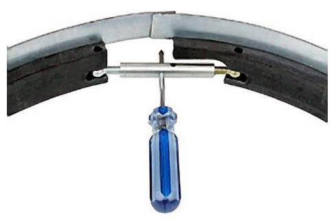
Our Manhole Adjusting Riser Rings feature a turnbuckle linkage pivoted at each end to provide the ultimate means to expand a manhole riser.
